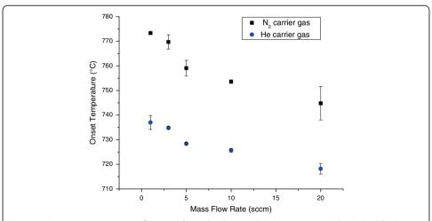
Figure 5 Onset temperature vs. flow rate for Iceland spar calcite ( $<53 \mu m$  particle size) with  $N_2$  (black squares) and He (blue circles) carrier gases. Higher flow rates (shorter evolved gas residence time) leads to lower decomposition temperatures for a particular carrier gas because the decomposition reaction takes place at a faster rate.
