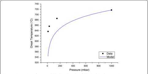
**Figure 2** Comparison of measured (black) and predicted (blue) calcite decomposition onset temperature at different pressures. Decomposition temperature clearly has a strong dependence on chamber pressure, and the shape of the model curve based on equilibrium thermodynamics matches laboratory measurements.
